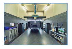
It also has an **internal metrology room** capable of issuing testing certificates, allowing it to be completely self-sufficient for everything related to the processing cycle and final testing of mechanical parts and molds.
